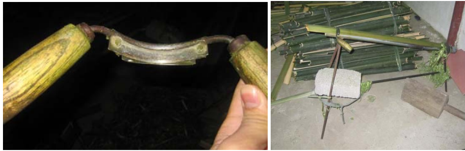
Figure 3. Newly designed graving knife (left) and graving manipulation (right)
