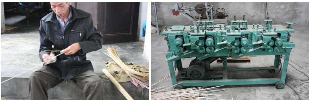
Figure 6. Manual splitting (left) and splitter (right)
