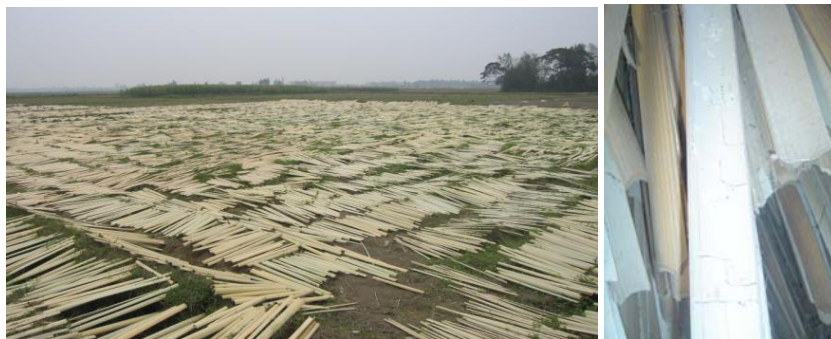
Figure 4. Drying material in the factory (left), moulded bamboo (right)
