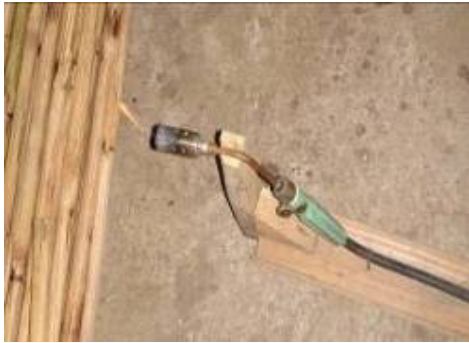
Figure 18. Gas driven curving equipment
