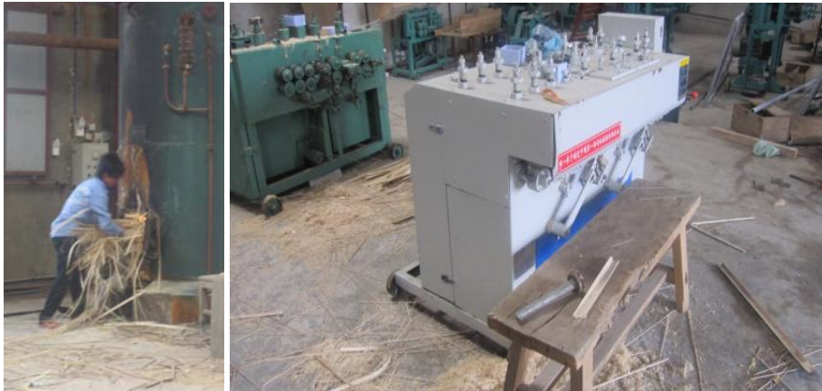
Figure 9. Utilising waste to fuel boiler (left) and produce tooth pick (right)
