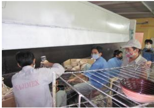
Figure 22. Spraying painting with air sucking and treating system
