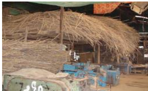
Figure 15. Preservation with classification and moisture insulation
